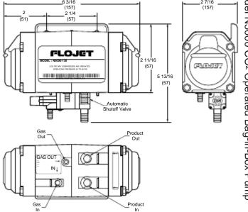
Product "OUT", use reinforced 1/2" (12.7 mm), 3/8" (9.5 mm) or 1/4" (6.3 mm) I.D. hose for discharge. Connect to product "OUT" port and dispensing head product (syrup) connection and clamp both ends securely.
